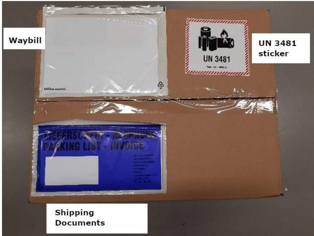
After the devices have been packed, place one printout of shipping documents and the return label (not visible on picture) on the outer side of box.
