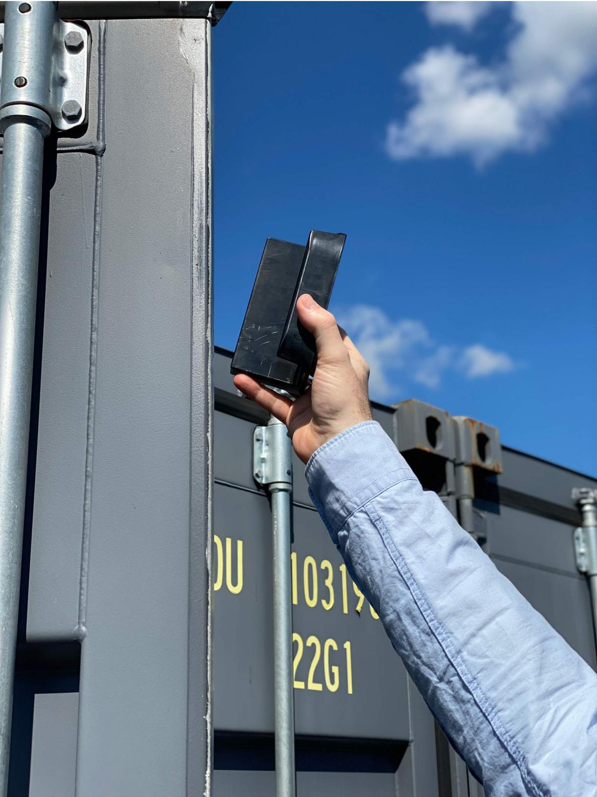
Mount the device on the container door **that has no rubber seal** on the side. This will usually be the left door.
