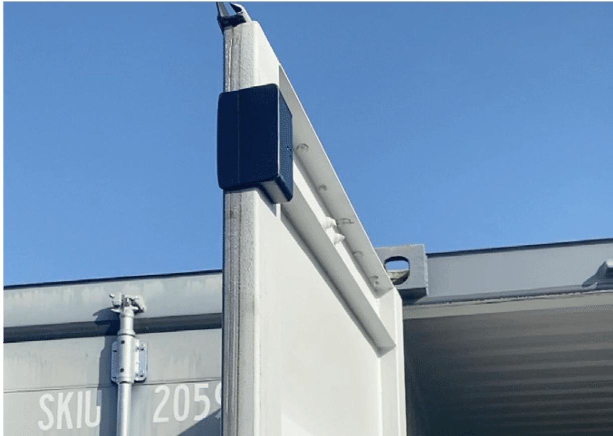
The device will be held in place by the in-built magnet.
